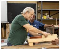
Jeff Bremer showed a wooden jointer plane he made. It has a fence and a Norris adjuster. He explained that he can clamp this plane upside down in a vice and use it to joint or plane small parts.
