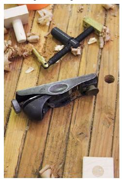
Steve said that you want to read the grain before starting to plane so that you do not lift the grain and get tear-out. You also want to transfer your pressure hand as you pass your plane across a cut, starting with downward pressure at the front of the plane and shifting that pressure toward the back of the plane as you finish the cut.
