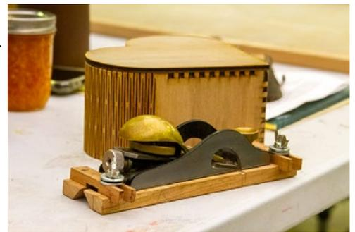
Calvin Sov presented a heart-shaped box he made using his CO<sub>2</sub> laser. It featured box joints and kerfing that allowed bent curves and was made from 1/4" Baltic birch plywood.
